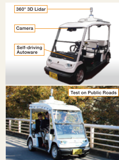
Slocal Self-driving System offers mobility to those that cannot drive and supports so called "last mile" transportation
