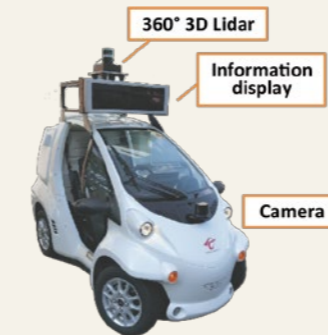
Slocal Self-driving System offers mobility to those that cannot drive and supports so called "last mile" transportation
