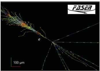
**Image title**: An electron neutrino detected by the FASERv detector at the LHC, the most energetic ever observed from a human source
